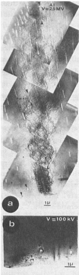
Fig. 7. Some area taken at 100 kV and 2.5 MV. The gain in penetration is about 10. Be fibres in the matrix of aluminium give an easy way to determine the penetration (ref. 12).
