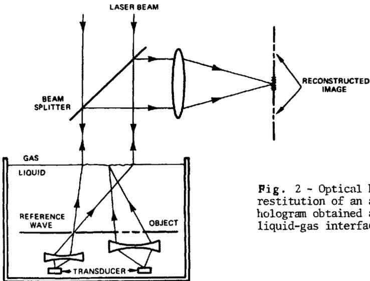
Fig. 2 - Optical holographic restitution of an acoustical hologram obtained at the liquid-gas interface.
