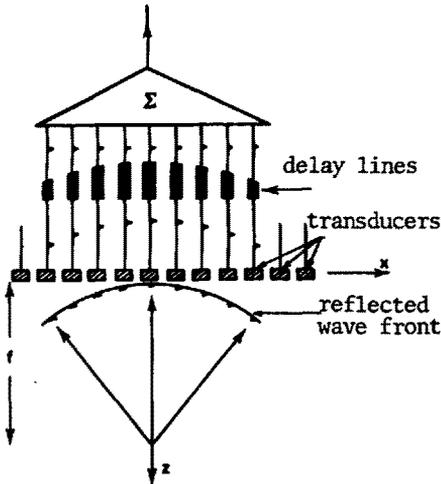
Fig. 5 - Electronic focusing during reception with delay lines.
