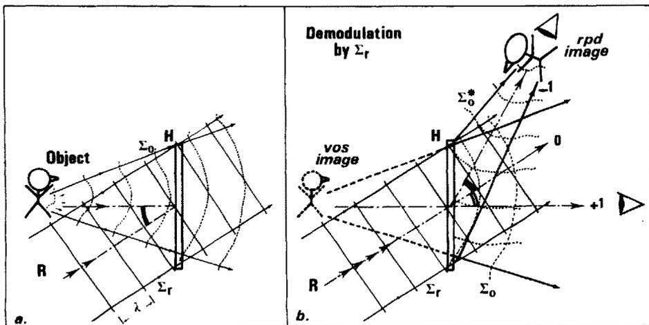
Fig. 1 : a - Recording set-up : R reference wave, O object, H : holographic plate (the dots indicate the emulsion),  $\Sigma_o$  object wave,  $\Sigma_r$  reference wave ;
