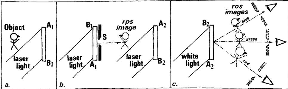
Fig. 3 : Principle of rainbow holography<sup>6</sup>. a - recording of a master hologram ; b - recording of a second hologram. The master hologram is illuminated by the conjugate reference beam (obtained by turning the hologram upside down) ; c - the reconstruction in white light yields polychromatic r, o, s images that are viewed through different "windows" - that prevent any color blurring.
