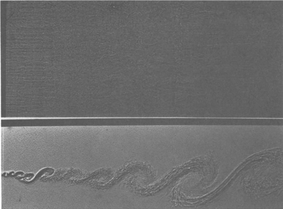
Fig. 2 Edge and plan views of a mixing layer
