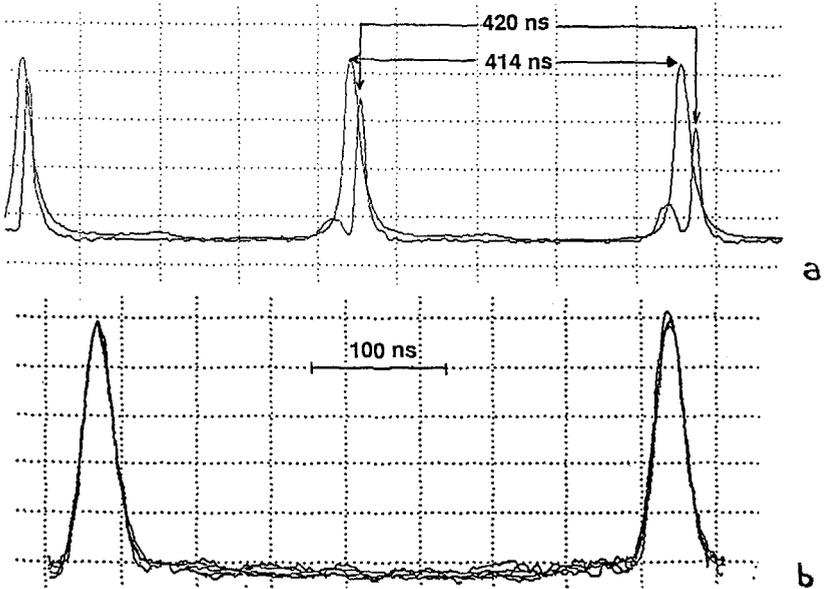
**Fig. 4** (a) Experimental superluminescent Brillouin Stokes solitons superimposed to the evolutive pulses spaced by  $\Delta t_L$ . (b) Experimental stability test of the Brillouin fiber-ring laser: six superimposed uncorrelated couples of pulses.
